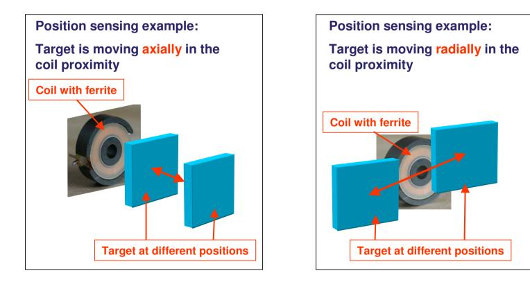
The wound coils as shown above are used up to 200 kHz excitation frequencies. They can be replaced by planar coils on the PCB or any substrate. Due to much lower inductances, planar coils should be driven at higher frequencies (typically 1 MHz to 2 MHz) to achieve high accuracy.
