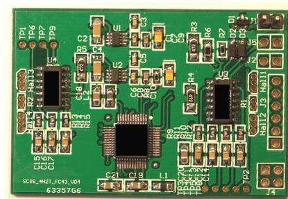
PCB example of a SCSS with SCI, JTAG and SPI interface for DC current sensing up to 800 A with bus bar 10 mm x 30 mm cross section.
