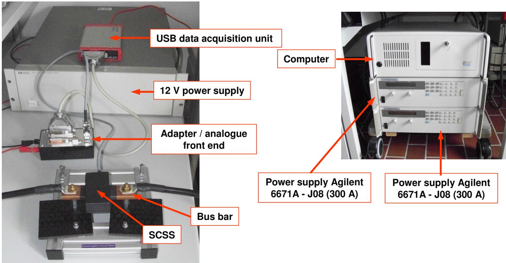
In addition to the standard bench test equipment, computer controlled power supplies (for max. 1.8 kA), data acquisition units and temperature chamber are currently available for SCSS tests.
