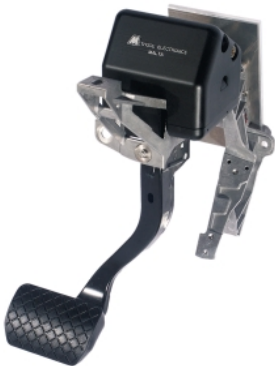
Figure 5: Prototype of the Brake Pedal Unit for EMB. The pedal sensor module and a passive pedal feel emulator are assembled in a pedal box, which is in series production at AUDI.
